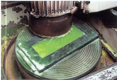
Surface grind of an oversized U core set on a vertical spindle CNC grinder
