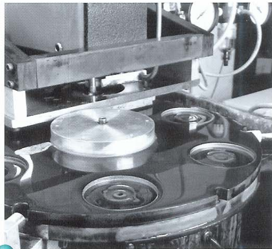
Automated gapping on Elna's CNC Robo-Gappers
