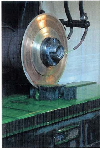
Slicing and slotting are performed on horizontal spindle CNC machines.
